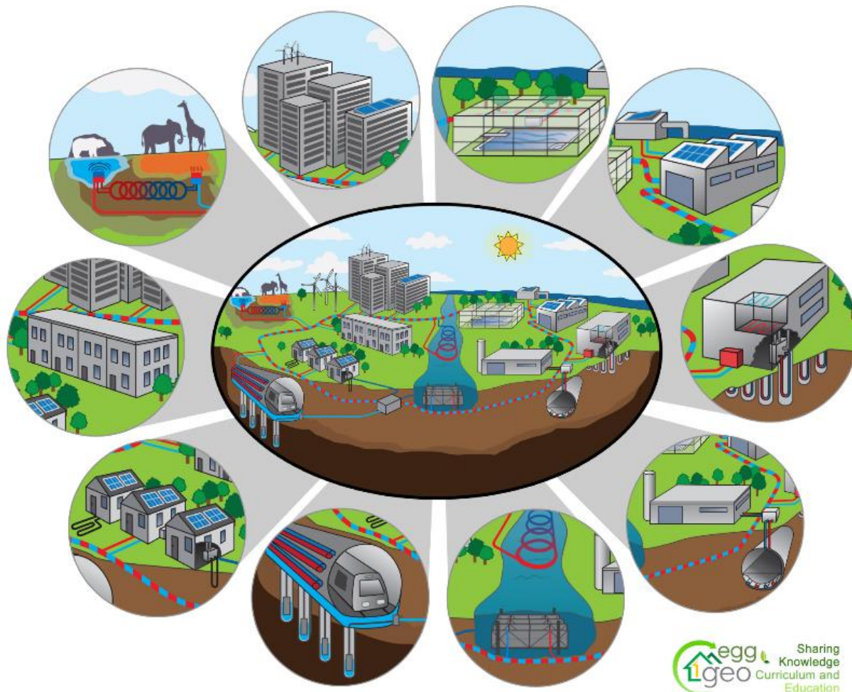
Figure 4: Some of the variations for heat sources and heat sinks in a District Geothermal Energy Network (Egg 2014)
